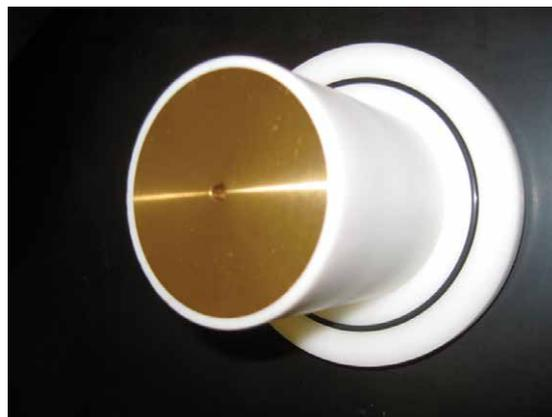
Figure 9: Acetal sensor mount showing annular lip that was machined flush with the insert (a brass insert is shown here).
