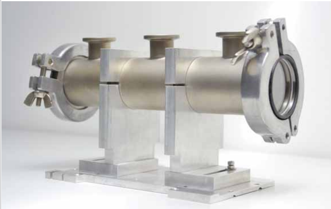
Stainless steel cylinder with sapphire-windows, 3 connection ports compatible to ISO KF 16
