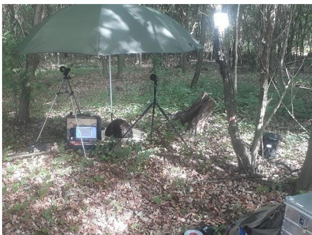
Figure 1: Setup of the measurement microphones
