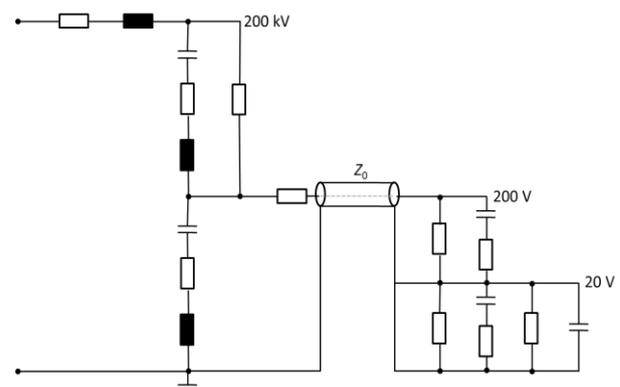
Figure 4 First design of a universal reference divider for superimposed voltages
