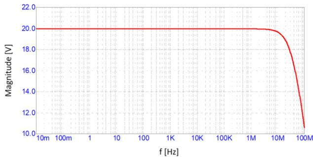
**Figure 5** Frequency response of the first design of a universal reference divider for superimposed voltages
