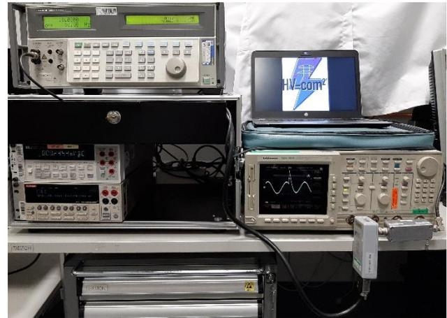
Figure 3 Low voltage generator for composite voltages
