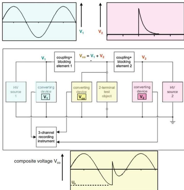
**Figure 2** Setup for composite voltages [7]
