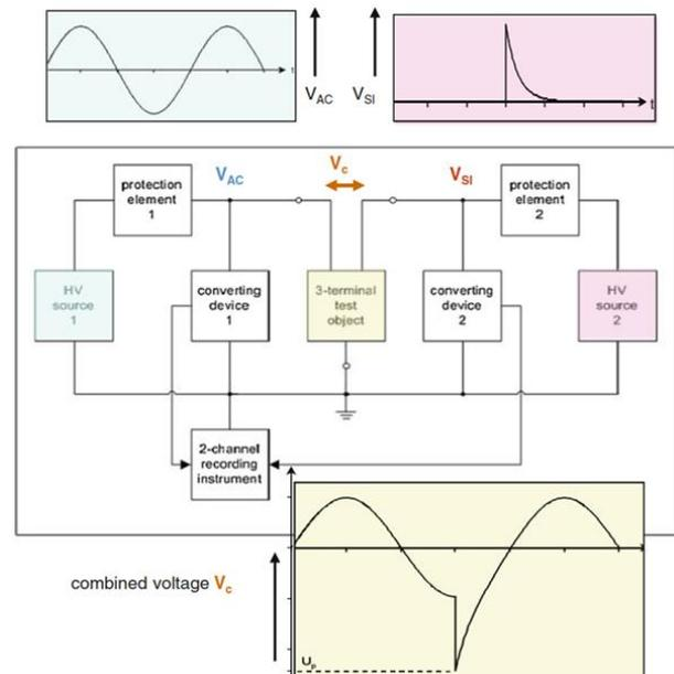
**Figure 1** Setup for combined voltages [7]
