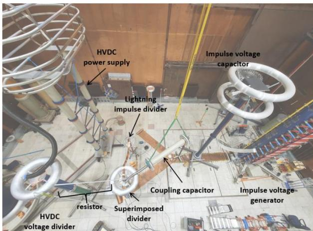
**Figure 6** Setup for superimposed voltage generation
