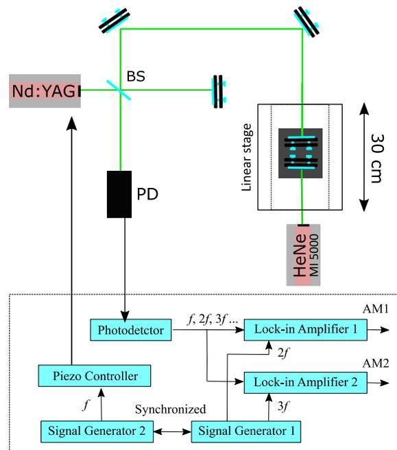
Figure 1. Experimental setup including a Beamsplitter (BS), Photodetector (PD).
