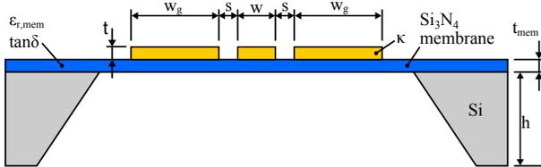
Fig. 2. Cross section of CPW built in membrane technology.
