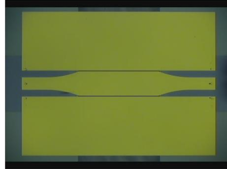
Fig. 1. Thru calibration standard fabricated in membrane technology.
