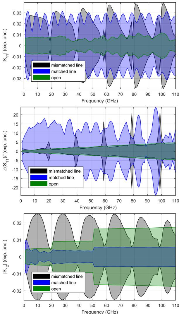
Fig. 5. Expanded uncertainty intervals at a coverage probability of 95% ( $k=2$ ).
