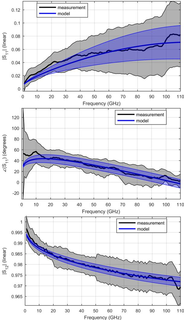
Fig. 4. Comparison between measured (black) and modeled (blue) reflection and transmission S-parameters of a 500  $\mu\text{m}$ -long matched line.
