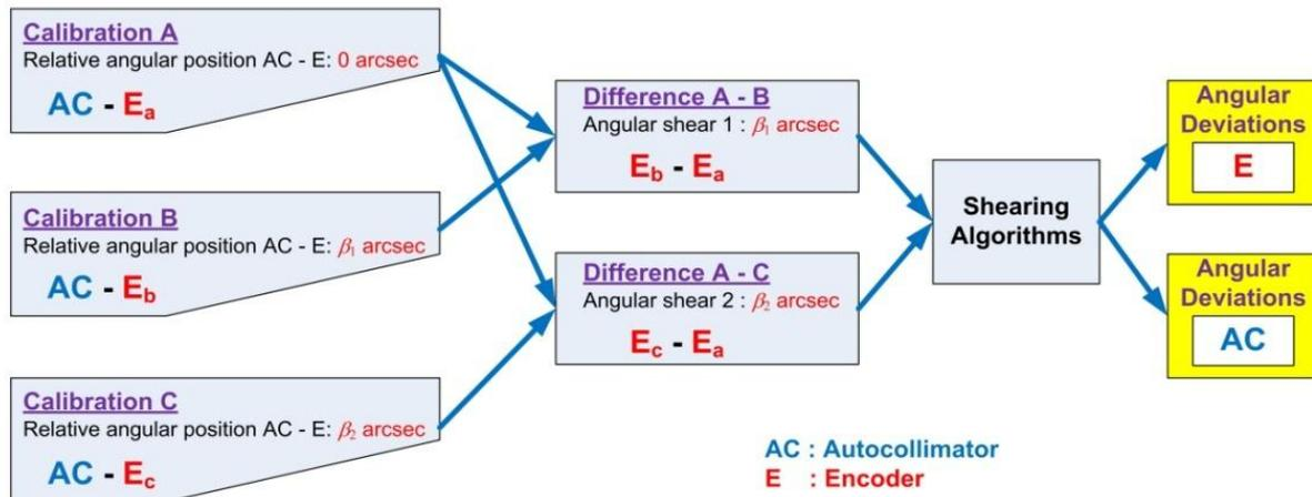
Figure 9: Schematic description of the shearing method.
