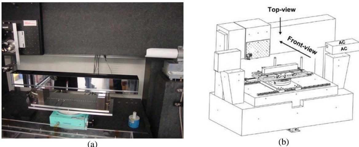
Figure 3: Autocollimator-based slope measuring profiler (NOM) of HZB (REG of SIB58 Angles), (a) Inspection of synchrotron radiation optics in HZB (b) Schematic view of NOM.
