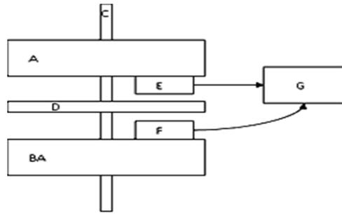
D continuously rotating optical encoder; F: reading head fixed to the reference frame BA; E: reading head fixed to the measuring table A; G: phase measurement
