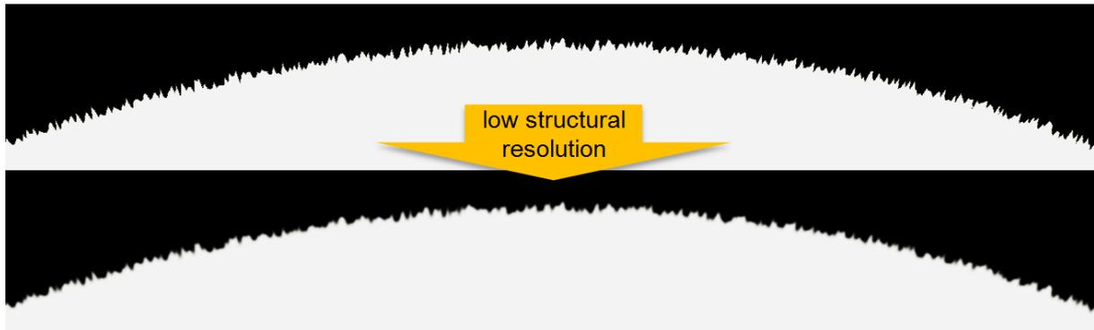
*Figure 1: Schematic illustration of the blurring effect of a CT measurement with limited structural resolution on volume data.*
