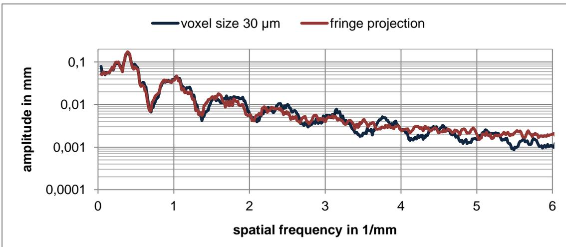
Figure 12: Measured amplitudes in comparison with a fringe projection system.
