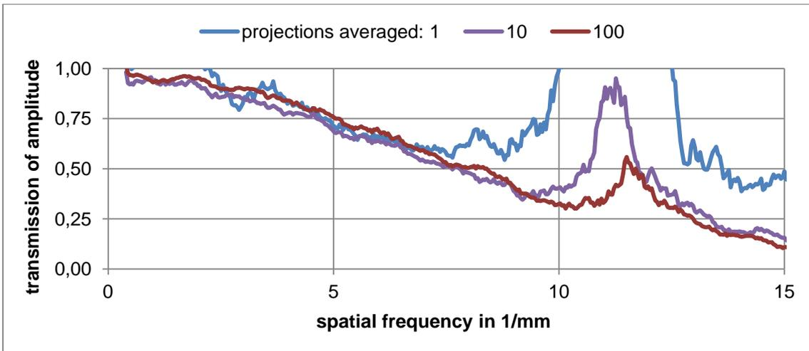
Figure 9: Simulated transmission of spatial frequencies for different settings of averaged projections.
