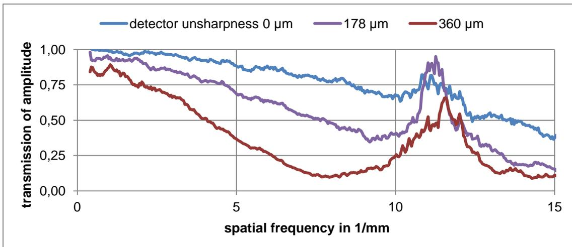
Figure 8: Simulated transmission of spatial frequencies for different settings of the detector unsharpness.
