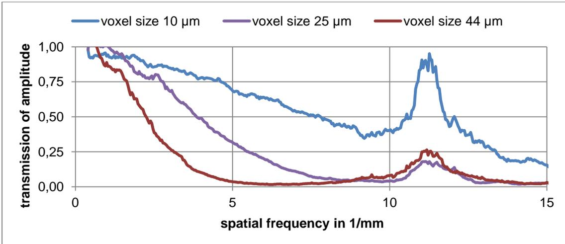
Figure 5: Simulated transmission of spatial frequencies for different geometrical magnifications.
