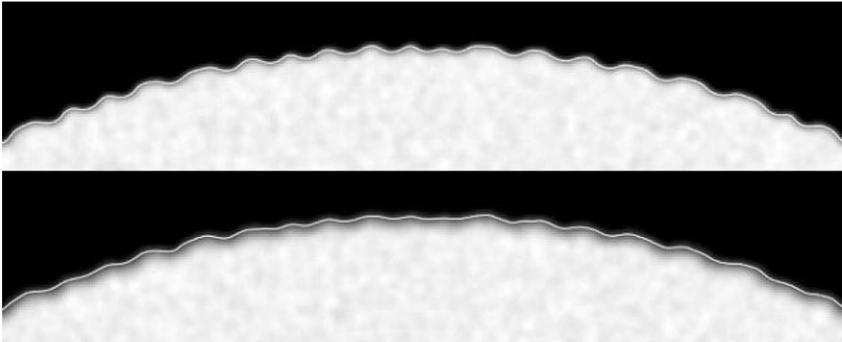
Figure 7: Comparison of simulated cross sections for spot sizes of 35  $\mu\text{m}$  (top) and 140  $\mu\text{m}$  (bottom). The white line indicates the extracted surface.
