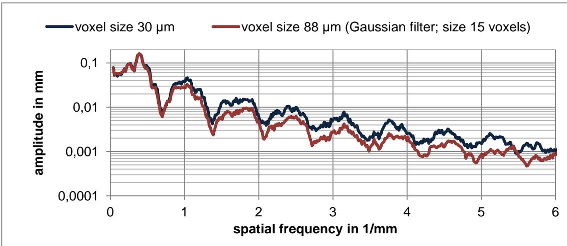
Figure 11: Measured amplitudes for different acquisition parameters.
