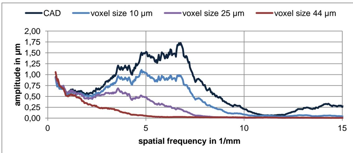
Figure 4: Simulated amplitudes for different geometrical magnifications.
