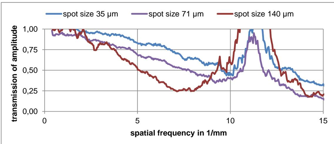
Figure 6: Simulated transmission of spatial frequencies for different X-ray spot sizes
