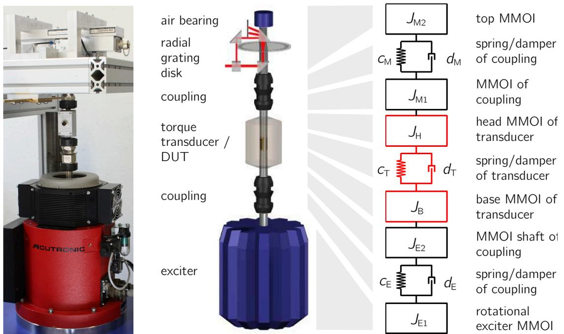
Figure 3: Dynamic torque calibration device (left), schematic image of corresponding components (middle) and model of the dynamic torque calibration device (right, black) including the model of the transducer (right, red).
