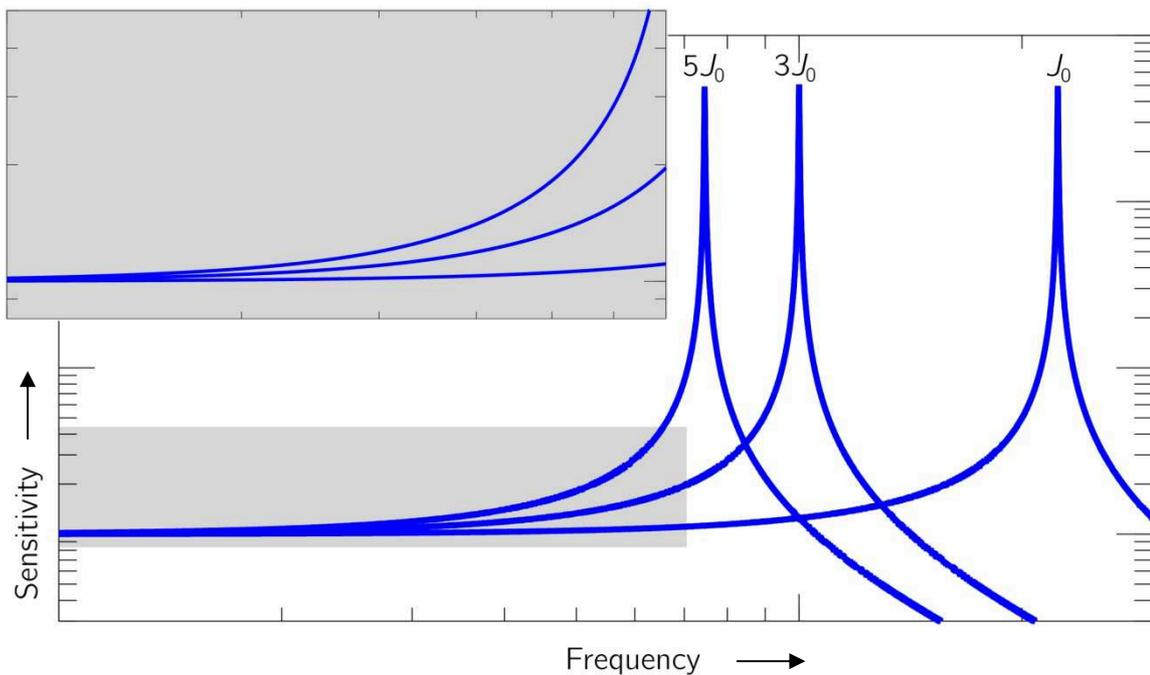
Figure 2: Frequency response of a transducer modelled as a SDOF system with different coupled MMOI resulting in a change of the frequency-dependent sensitivity.
