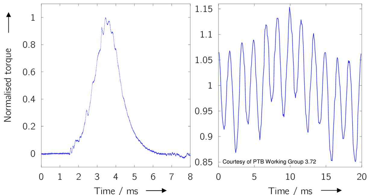
Figure 1a: Fastening cycle of an impulse wrench (left).
