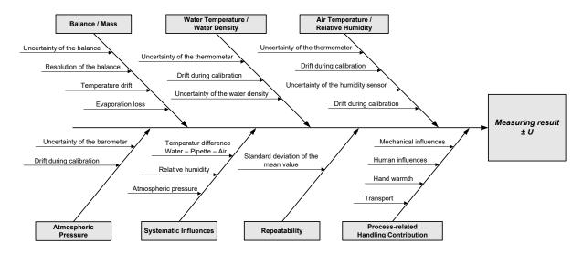
**Figure 1:** Influences on the measurement uncertainty during the calibration of piston-operated pipettes
