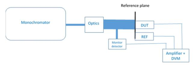
Fig. 3. Responsivity measurement setup
