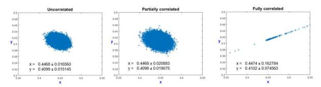
**Fig. 7.** left: Correlation due to overlapping colour-matching functions and with no additional correlation within the measurement process of the spectral data; centre: with additional partially correlated measurement procedure of the spectral data; right: with additional full correlation of all the spectral data. Note: The uncertainty of the wavelength scale calibration leads to a shift of the spectral points which does not cancel out in x and y.
