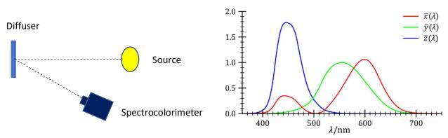
Fig. 5. Left: Measurement setup; Right: CIE 1931 XYZ Color Matching Functions
