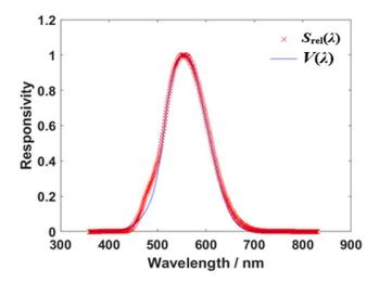
Fig. 8. Relative spectral responsivity  $s_{\rm rel}(\lambda)$  of the studied photometer and  $V(\lambda)$  curve in the wavelength range 360 nm - 830 nm. The photometer quality index  $f_1$ ' is 7.3 %.
