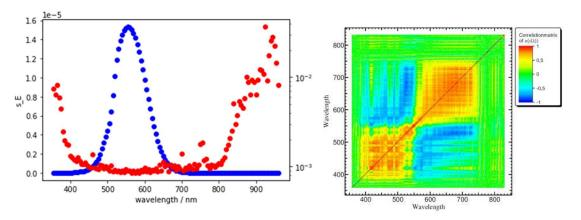
**Fig. 4**. <u>Left:</u> spectral irradiance responsivity (blue; left axis) and the relative standard uncertainty (red; right axis) of a photometer; <u>Right:</u> the corresponding correlation matrix [14]
