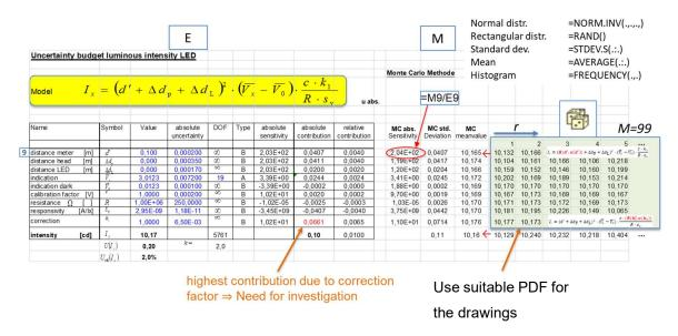
**Fig. 1.** EXCEL-based example for determination of sensitivity coefficients and measurement uncertainty for the Averaged Luminous Intensity Type B (see CIE 127) [8]. The values in blue are input values for the MC calculation of the combined uncertainty
