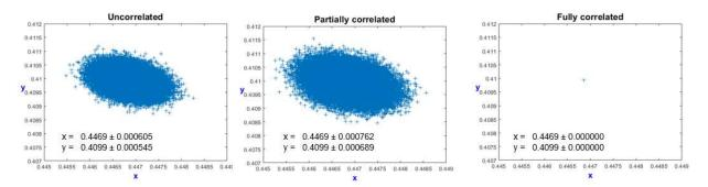
**Fig. 6.** left: Correlation due to overlapping colour-matching functions and with no additional correlation within the measurement process of the spectral data; centre: Additional partial correlation due to the measurement procedure of the spectral data; right: Additional full correlation of all the spectral data. *Note:* The uncertainty of the reflection calibrations leads to an amplitude shift, which is cancelled out in the ratio of Eq. 40 if the correlation is complete.
