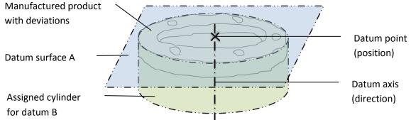
Figure 8 Datum assignment at the manufactured flange.
