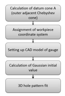
Figure 19 Flowchart for 3D hole pattern fit for a conical disk.
