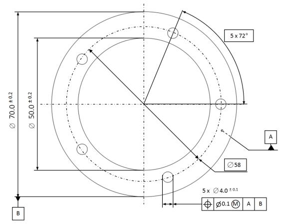
Figure 7 ISO 1101 compliant inspection of the flange.
