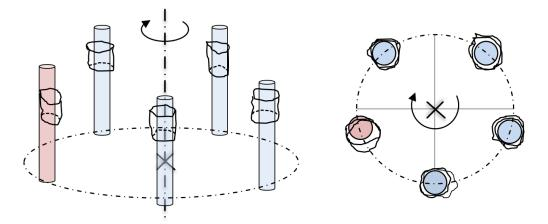
**Figure 9** 3D hole pattern fit for the flange (on the left: perspective view, on the right: top view); the gauge cylinder highlighted in red overlaps with the hole. By rotating all gauge cylinders around the datum axis, no position is found where all cylinders lie within the holes.
