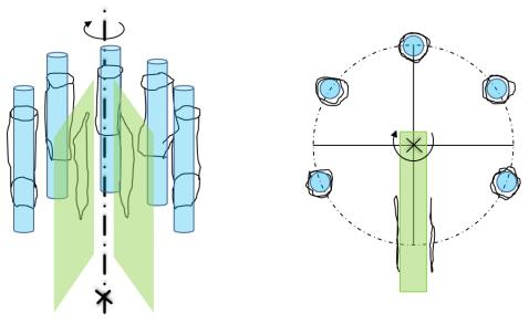
Figure 18 3D hole pattern fit for the conical disc.
