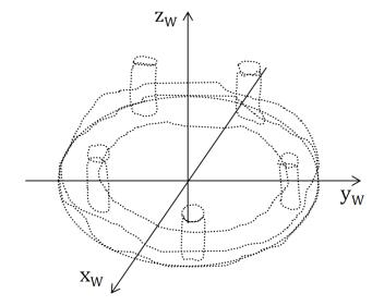
Figure 11 Workpiece coordinate system and extracted geometry at the flange.
