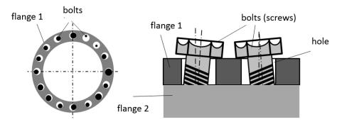
Figure 1 Outline of the assembly requirements for a flange connection with a bolt.
