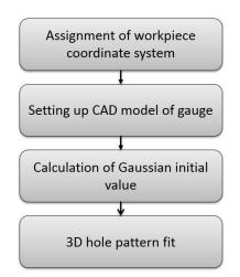
Figure 24 Flowchart on the 3D hole pattern fit for the cube.
