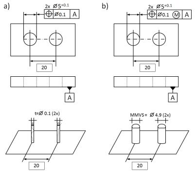
**Figure 2-1** Two examples for tolerancing a plate with two holes. The virtual inspection of the tolerances presupposes the 3D hole pattern fit in both cases (Tolerance principle ISO 8015).
