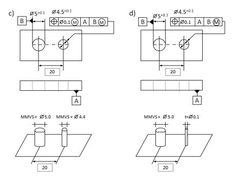
Figure 2-2 Tolerances with datum features including drawing specifications ®.
