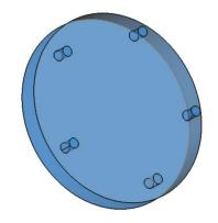
Figure 13 Counterpart for flange assembly.
