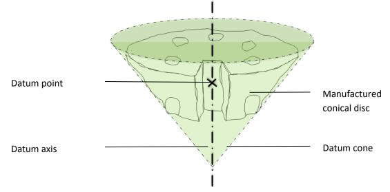
Figure 17 Datum assignment at the manufactured conical disc.
