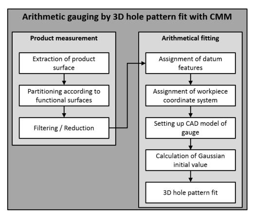
Figure 3 Principal procedure of the arithmetic gauging by means of coordinate measurement machines.
