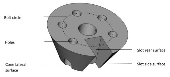
Figure 15 Example of a conical disc
