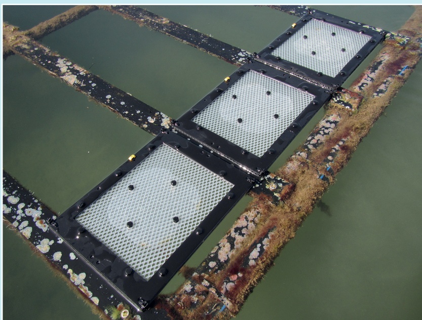
Fig. 5: Metal mesh with samples attached to it in the Mediterranean Sea
