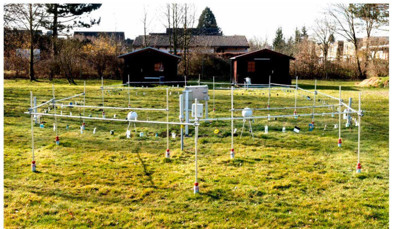
Figure 1: Photograph of the ERADOS during an intercomparison of passive H^*(10) area dosimeters for environmental monitoring
