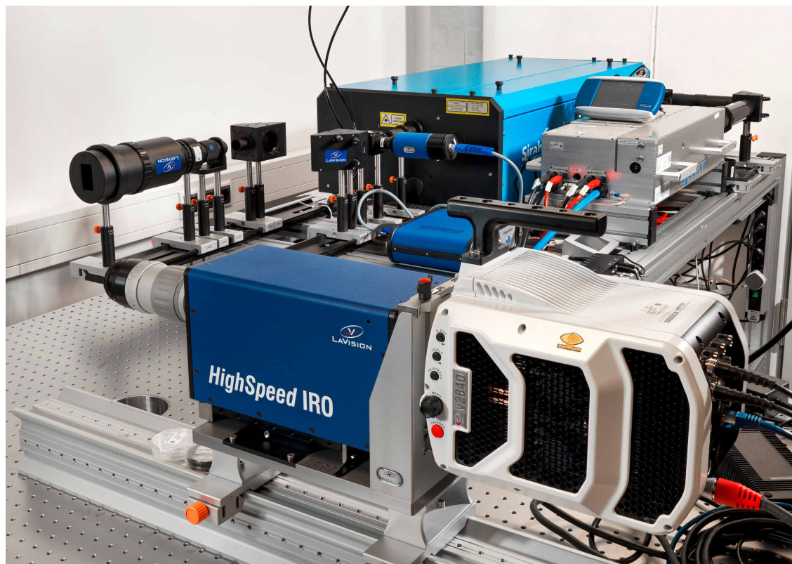
Figure 8: High-speed laser induced fluorescence facility used to investigate ignition processes of hydrogen mixtures such as turbulent hot jet ignition
