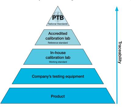
Figure 3: Calibration hierarchy in the Federal Republic of Germany.
