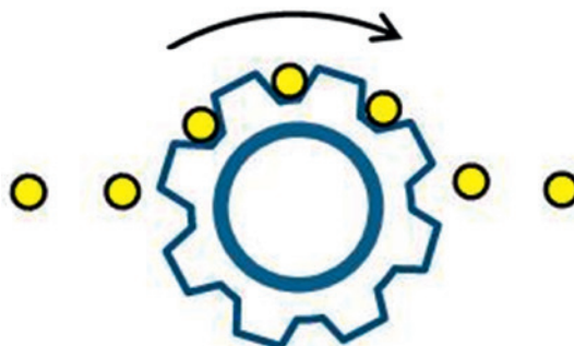
Fig. 4: Illustration of the principle of a single-electron current source, depicted as a gear for the clocked transport of single electrons (charge quanta, yellow). In each recess between two neighboring “teeth”, one electron is transported.
