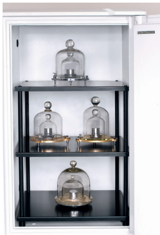
Figure 5: Held in safekeeping – PTB holds several prototypes of the kilogram, such as the two specimens issued to the Federal Republic of Germany (#52, top level in safe) and the German Democratic Republic (#55, middle left) in the early 1950s, as well as an additional prototype (#70, middle right) acquired by the Federal Republic of Germany in 1987. Kilogram number 22 (lower level in safe) is from 1889, was damaged during war-time and is no longer an official prototype.
