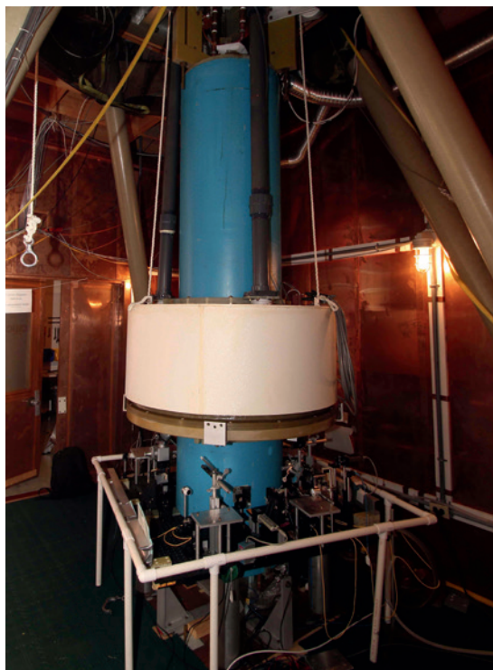
Figure 9: The NIST watt balance, lower level. In the blue cylinders, there are the superconducting magnetic coils, in the white ring there are the induction coils, the latter being in vacuum. (Photo: by the author)
