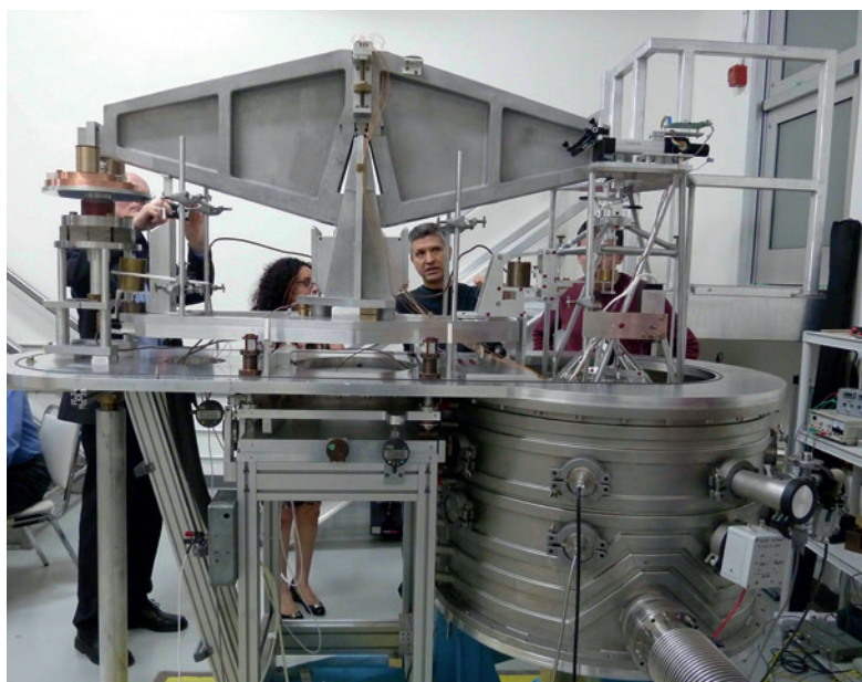
Figure 7: The NRC watt balance, vacuum lid raised. (Photo: by the author)
