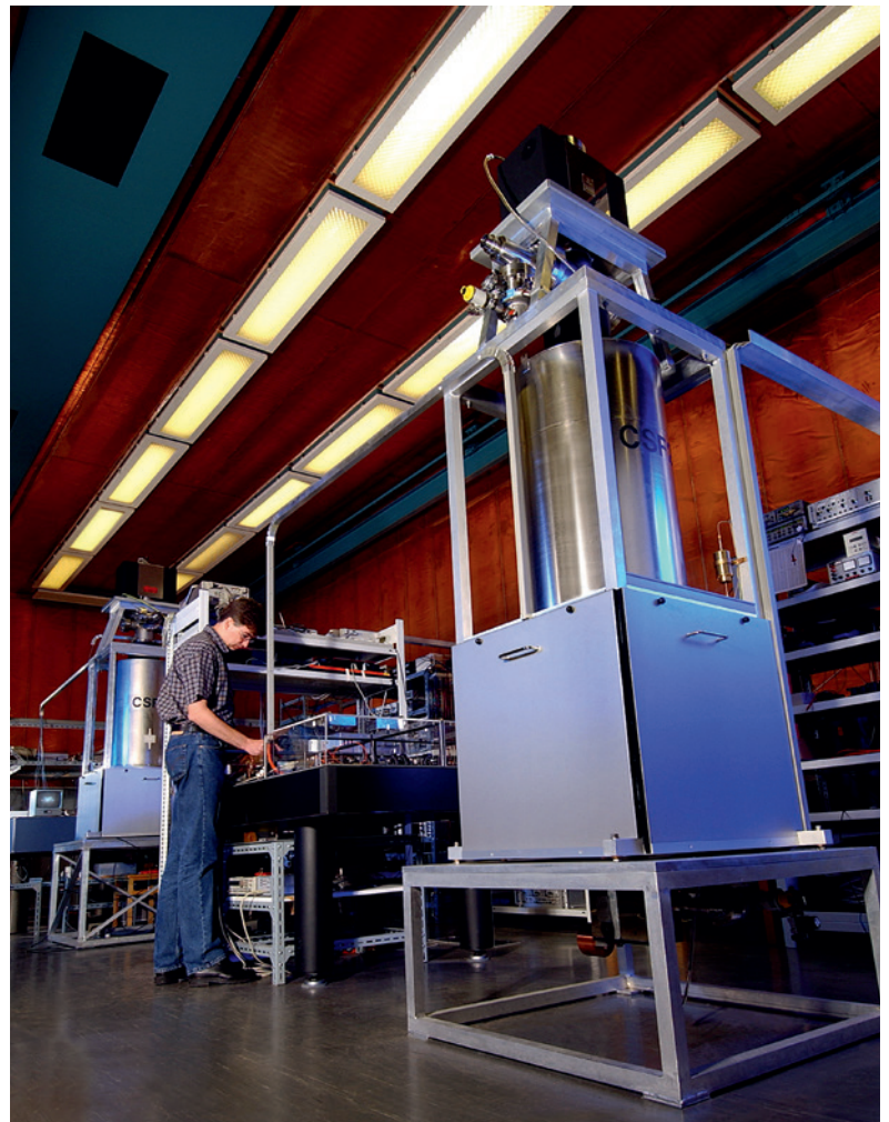
Figure 5: PTB's cesium fountain clocks CSF1 (in the background) and CSF2 (in the foreground) in 2005.
