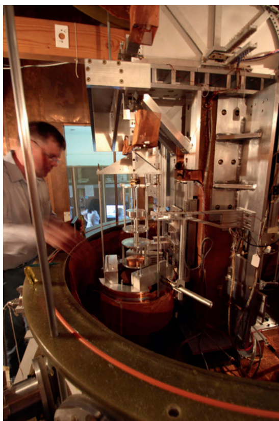
Figure 10: The NIST watt balance, upper level with open vacuum bell jar, in the middle there is the suspension with the weight exchange facility for the weight. The cable pulley is located further up. (Photo: by the author)
