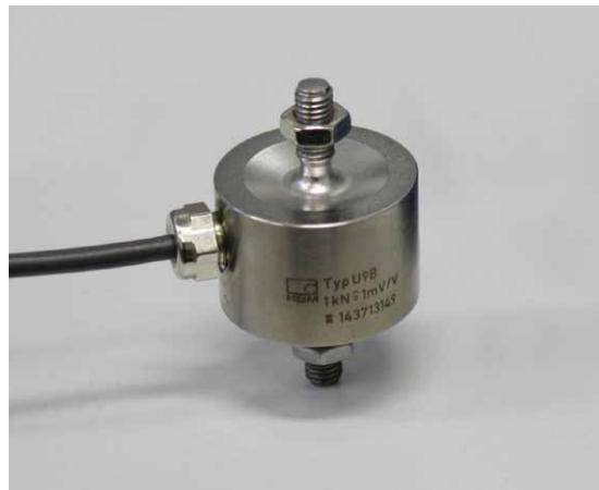
HBM U9B as an example of investigated force transducers in the project.
