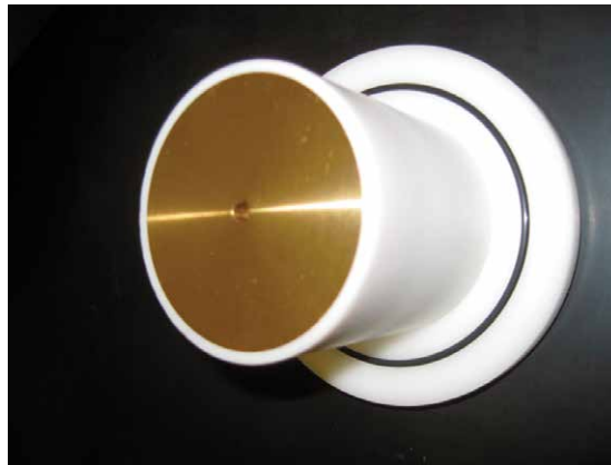
Figure 9: Acetal sensor mount showing annular lip that was machined flush with the insert (a brass insert is shown here).
