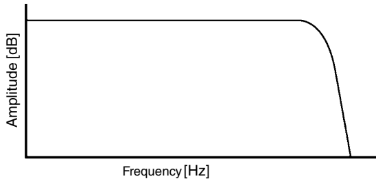
Needed frequency response of a bridge amplifier.
