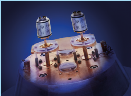
Calorimeter for the calibration of HF power thermistors
