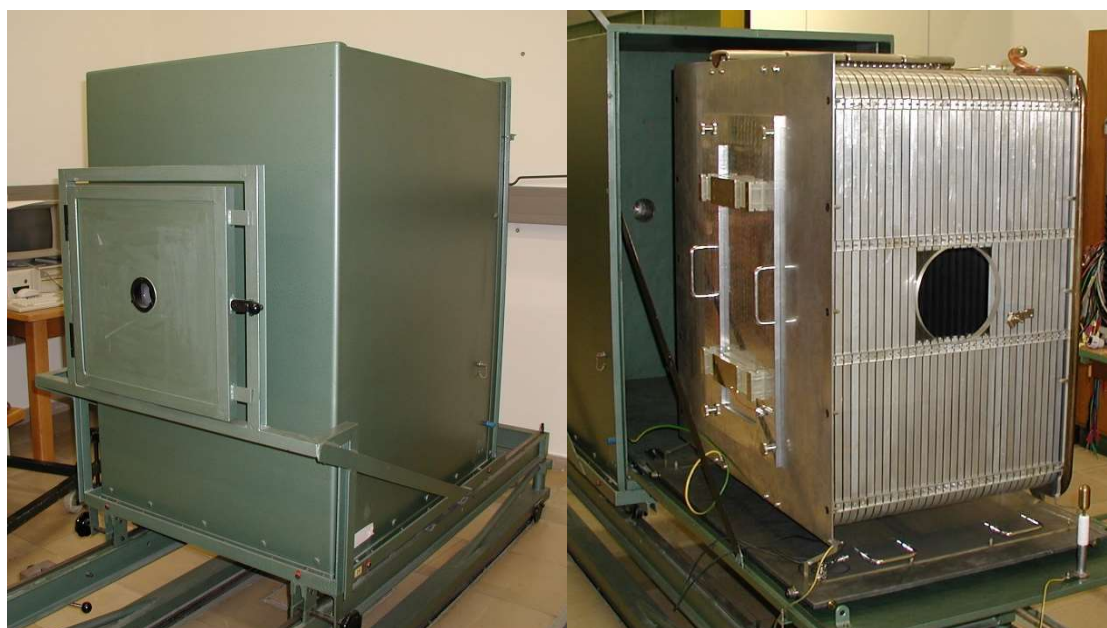
Figure 33. Photo of the free-air chamber type PK400 with (left) and without (right) its lead housing.
