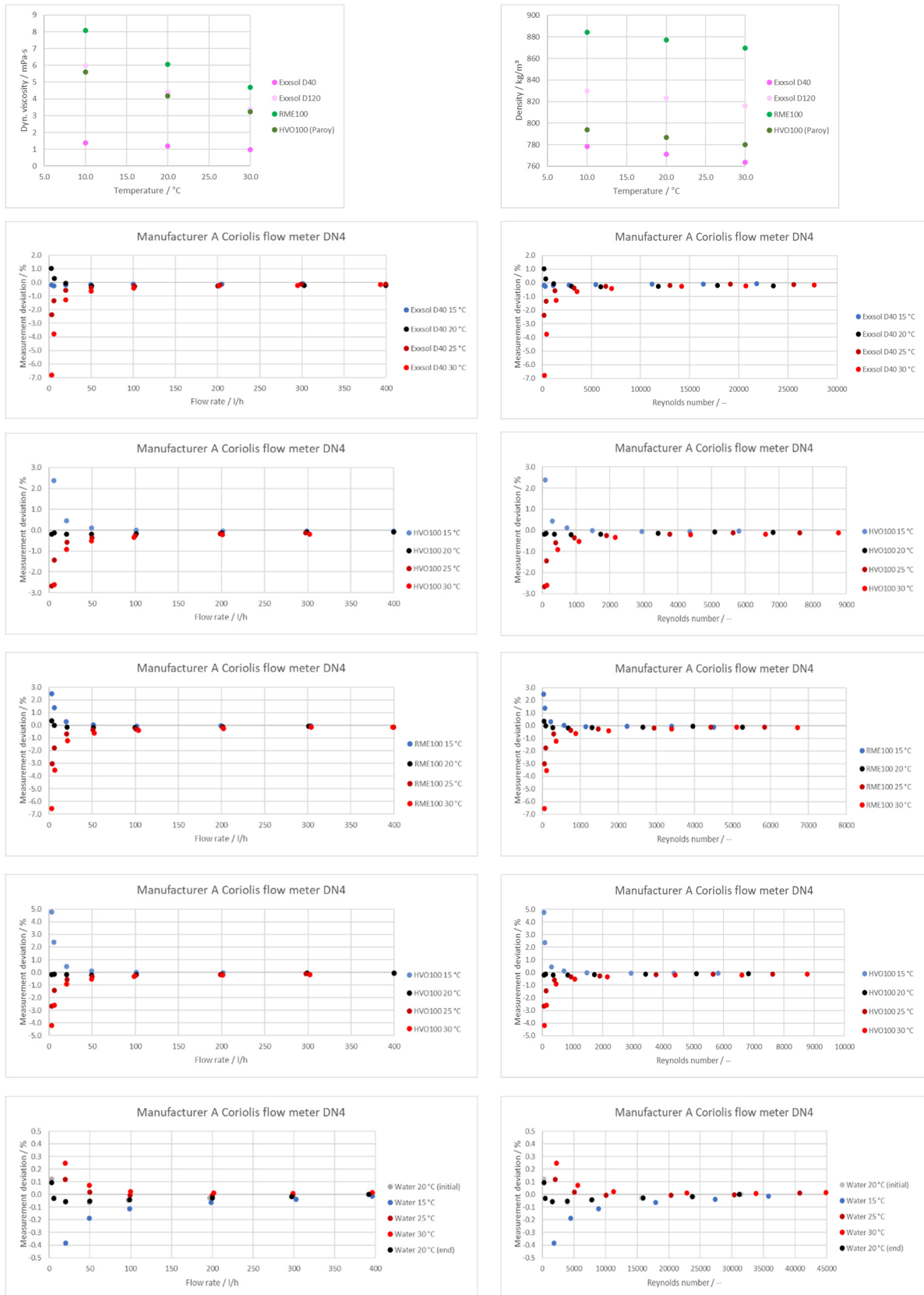
Fig. 11. Measurement deviations and Reynolds numbers of a Coriolis flow meter (pulse value: 60000 p/kg resp. 60000 p/l) for different types of liquids and at different liquid temperatures. Partly different scaling of x- and y-axes. Top: Temperature-dependent dynamic viscosity and density of the hydro-carbon test liquids.
