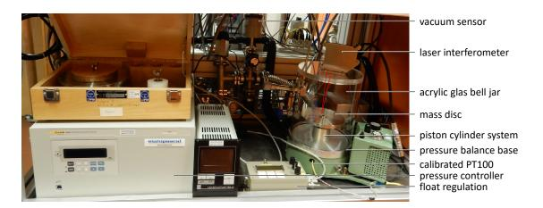
Figure 4.10.: The automated pressure balance and its main components used for the calibration of the digital pressure sensors.
