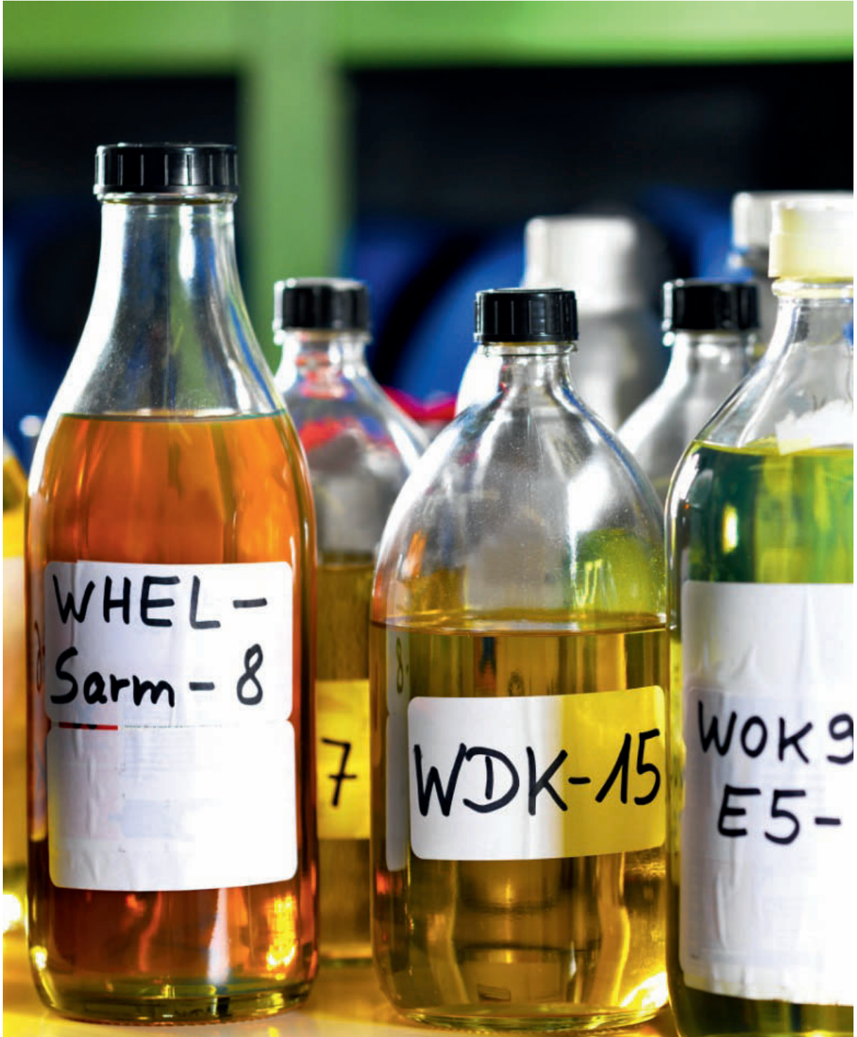
Fuel samples gathered throughout Germany to measure the transport quantities "density" and "viscosity"
